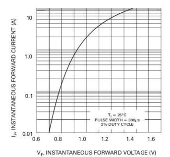
Fig. 2 Typical Forward Characteristics
