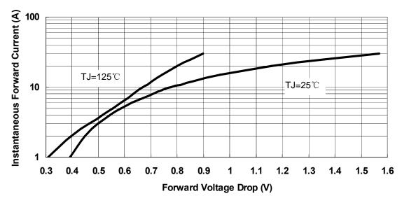
Fig.3-Typical Instantaneous Forward Voltage Characteristics
