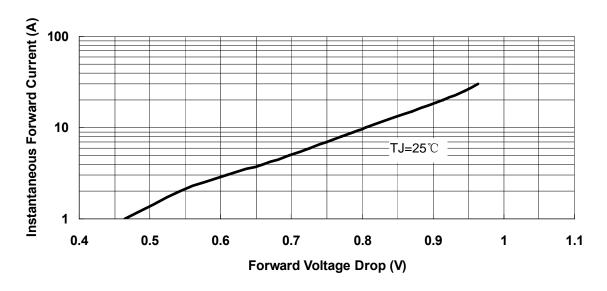
Fig.3-Typical Instantaneous Forward Voltage Characteristics
