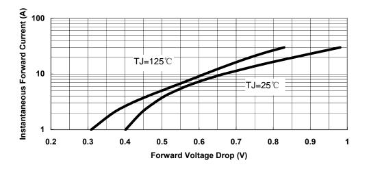
Fig.3-Typical Instantaneous Forward Voltage Characteristics
