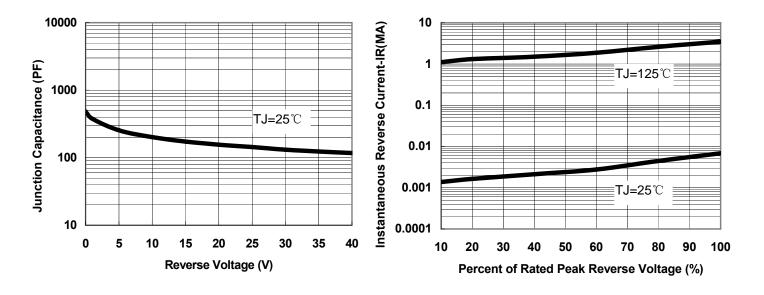
Fig.1-Typical Junction Capacitance
