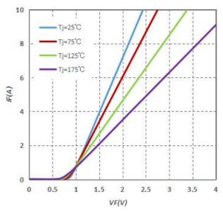
Fig.1-Typical Forward Voltage Characteristics
