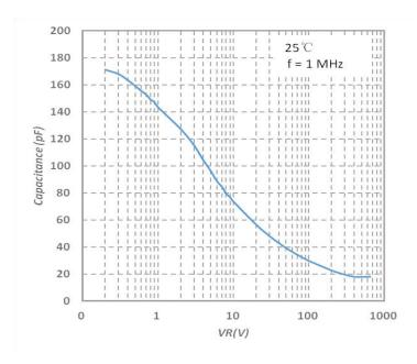
Fig.3-Capacitance vs. Reverse Voltage
