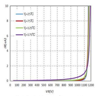
Fig.2-Typical Reverse Characteristics
