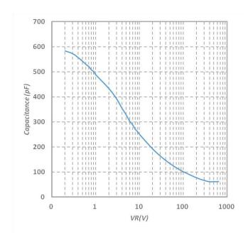
Fig.3-Capacitance vs. Reverse Voltage
