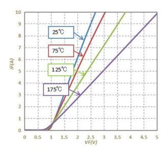
Fig.1-Typical Forward Voltage Characteristics
