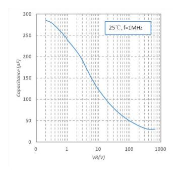
Fig.3-Capacitance vs. Reverse Voltage
