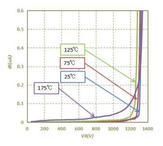
Fig.2-Typical Reverse Characteristics
