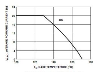
FIGURE 3.CURRENT DERATING CURVE
