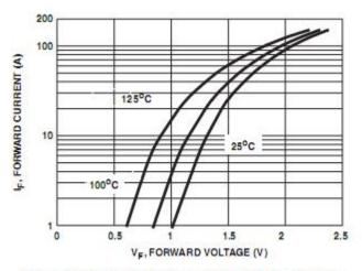
FIGURE 1. FORWARD CURRENT VS FORWARD VOLTAGE
