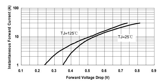
Fig.3-Typical Instantaneous Forward Voltage Characteristics
