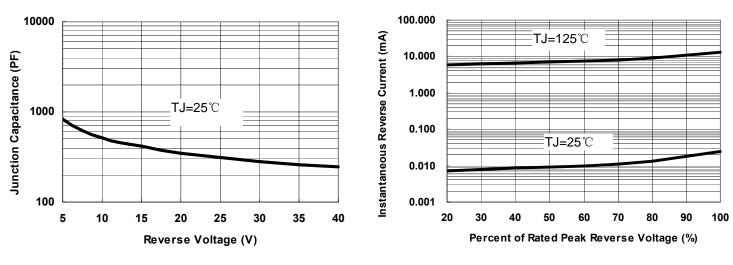
**Fig.1-Typical Junction Capacitance**
