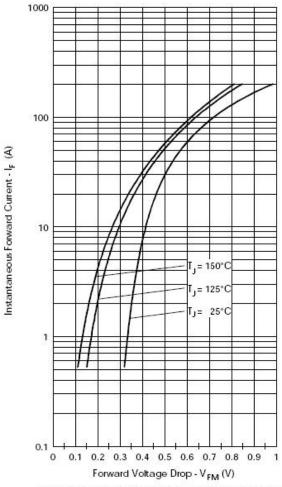
Fig. 1-Maximum Forward Voltage Drop Characteristics
