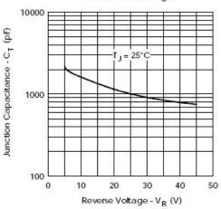
Fig. 3-Typical Junction Capacitance Vs. Reverse Voltage
