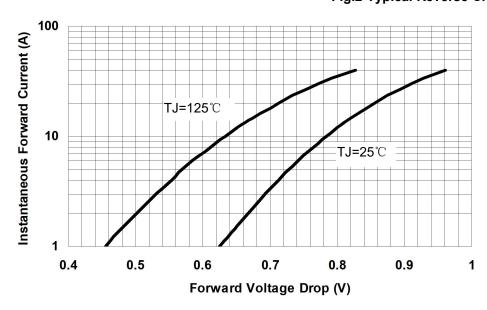
Fig.3-Typical Instantaneous Forward Voltage Characteristics
