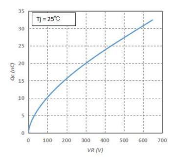
Fig.4-Total Capacitance Charge vs. Reverse Voltage
