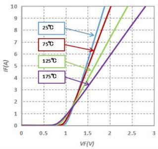
Fig.1-Typical Forward Voltage Characteristics
