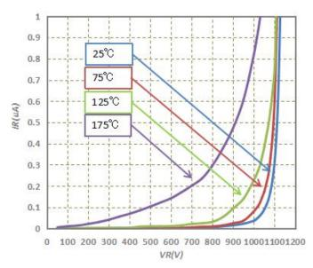
Fig.2-Typical Reverse Characteristics
