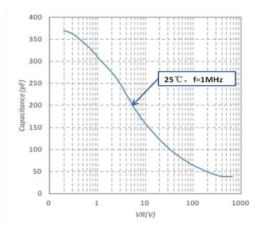
Fig.3-Capacitance vs. Reverse Voltage
