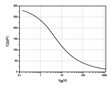
Fig.3-Capacitance vs. Reverse Voltage
