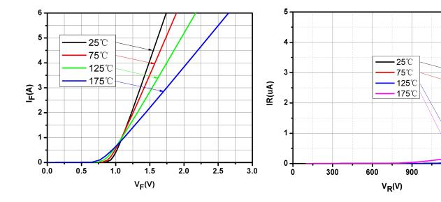
Fig.1-Typical Forward Voltage Characteristics
