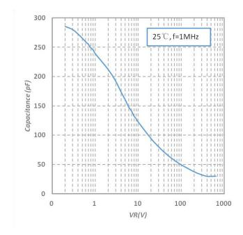
Fig.3-Capacitance vs. Reverse Voltage
