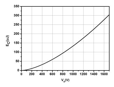
Fig.7-Capacitance Stored Energy
