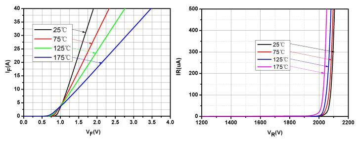
Fig.1-Typical Forward Voltage Characteristics
