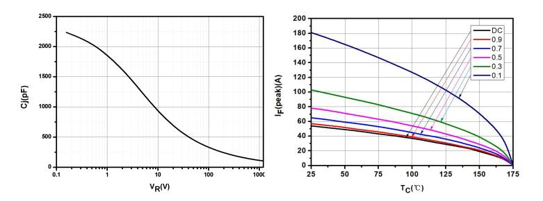
Fig.3-Capacitance vs. Reverse Voltage
