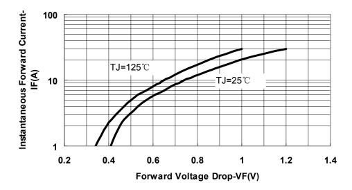
Fig.3-Typical Instantaneous Forward Voltage Characteristics
