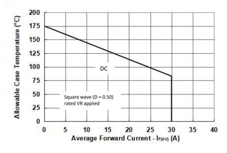
Figure 12 Maximum Allowable Case Temperature vs.
