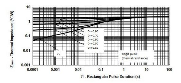
Figure 13 Typical Thermal Impedance ZthJC Characteristics
