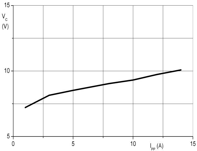
Fig 4. Clamping voltage as a function of peak pulse current
