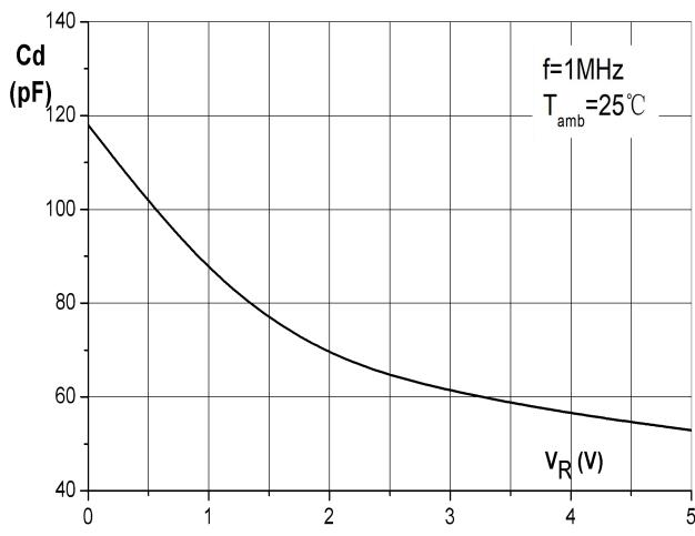
Fig 3. capacitance as a function of reverse voltage
